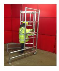
2) OPEN FRAME AND LOCK MECHANISM
